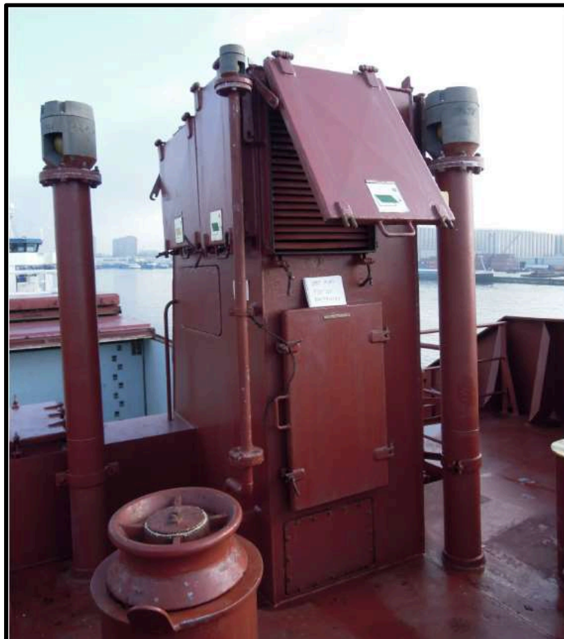
Fig 11: Location of Ford Ventilators
