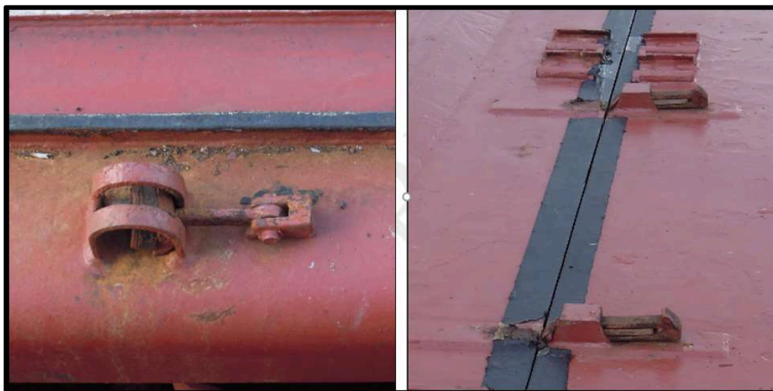
Fig 31 Hatch Covers – Dogs and Cleats
