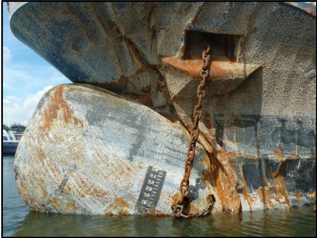
Fig 36 Damage to Bulb section
