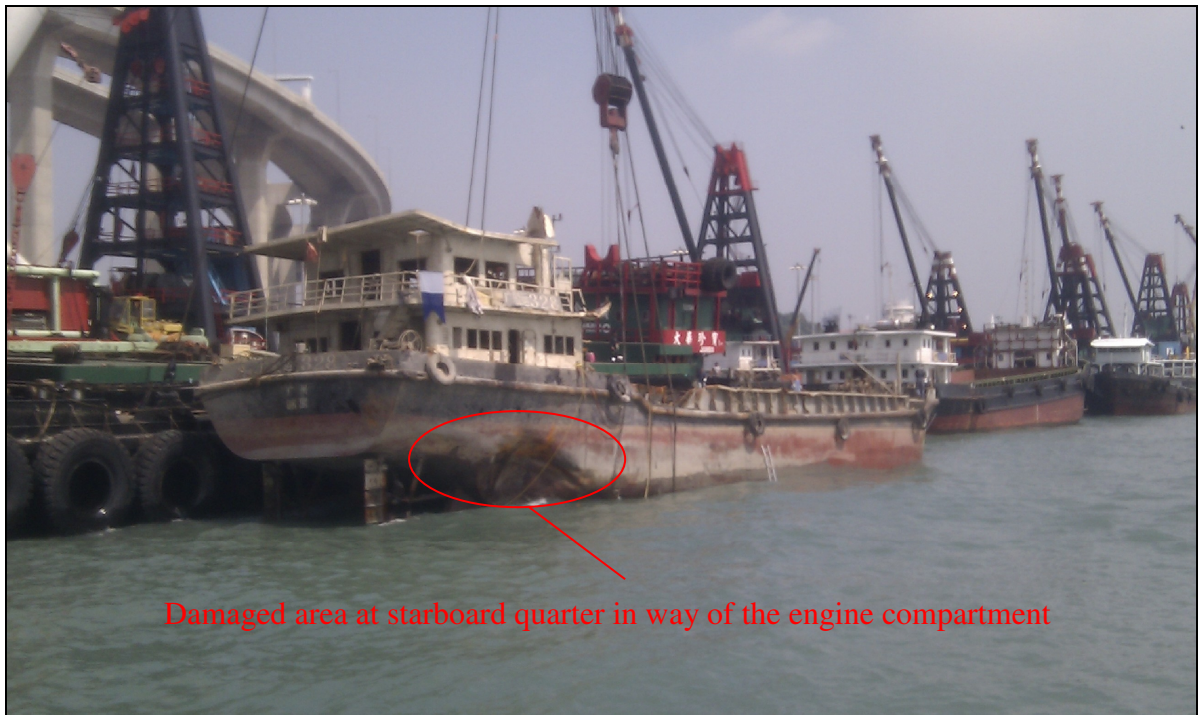
Figure 3b – GUANG BO YUN 328 secured alongside a berth after being salvaged and temporarily repaired.
