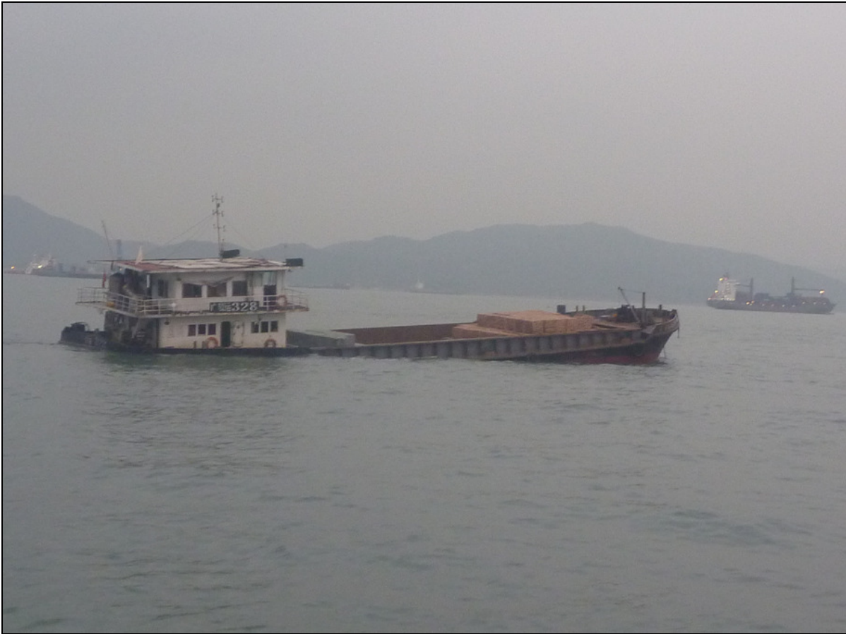
Figure 3a – GUANG BO YUN 328 sank by the stern and slightly listed to starboard after the collision, and finally foundered in about 2 hours.
